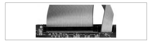
If you have two DB-15 connectors on your cable adapter bracket, you should attach the flat ribbon cables of the dual DB-15 connectors to the top internal auxiliary I/O 32-pin connector.
