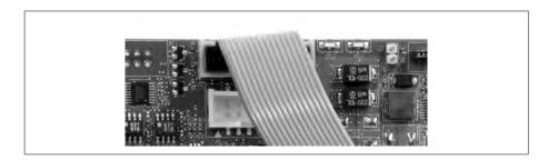
If you have DB-44 and DB-9 connectors on your cable adapter bracket, you should attach the flat ribbon cable of the DB-44 connector to the internal auxiliary I/O 44-pin connector and you should attach the flat ribbon cable of the DB-9 connector to the internal auxiliary 10-pin connector.
