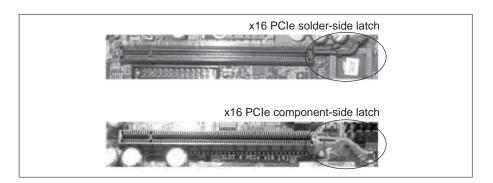
The PCIe specification does not define appropriate keep-out regions for the latch to provide any tolerance to tilting or rotation when inserting or removing add-in boards in these connectors. Therefore, do not to tilt the Matrox Solios eV-CL
