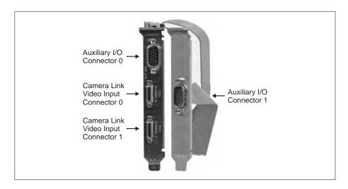
To Matrox Solios eV-CLB in dual-Base configuration, you can connect two independent video sources; one to each Camera Link connector. To Matrox Solios eV-CLB in single-Medium configuration and to Matrox Solios eV-CLF, you can only connect a single video source, regardless of the source's configuration.
