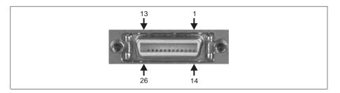
The pinout of these connectors follow the Camera Link standard, and are identical to the pinout of the corresponding connectors on Matrox Solios eV-CLB and Matrox Solios eV-CLF described earlier in this appendix.
