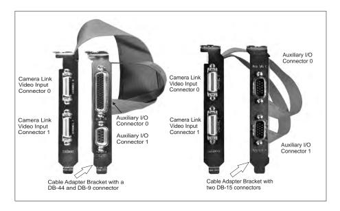
To Matrox Solios eV-CLBL in dual-Base configuration, you can connect two independent video sources; one to each Camera Link connector. To Matrox Solios eV-CLBL in single-Medium configuration and to Matrox Solios eV-CLFL, you can only connect a single video source, regardless of the source's configuration.
