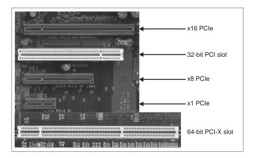
Matrox Solios eV-CL might drop frames if there are not at least 4 active lanes on the PCIe connector to the Host (for example, if the board is connected to a x4 PCIe connector that has only one active lane). Verify with your motherboard manufacturer to find out whether your motherboard works efficiently with a x4 PCIe board, such Matrox Solios eV-CL.
