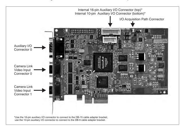
On the cable adapter bracket, there is another external auxiliary I/O connector (DB-15 or DB-9); this allow you to access the signals of the internal auxiliary I/O connectors from outside the computer enclosure.
