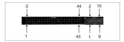
The pinout for internal 44-pin auxiliary I/O connector is as follows. Refer to the description of external auxiliary I/O connector 1 to establish if an auxiliary signal is specific to an independent acquisition path and the type of signals that can be routed onto it.
