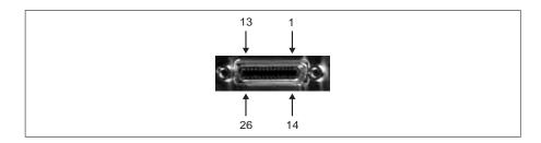
For Matrox Solios eV-CLB in dual-Base configuration, the two Camera Link video input connectors have the same pinout; this pinout is listed in the following table. Note that, in dual-Base configuration, each connector supports video input from a different video source.
